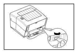
**IMPORTANT:** If you install the *Toner Container* and switch on the power, two indicators will start fast flashing. When the printer is first switched on after toner installation, there will be a delay of approximately 15 minutes before the printer gets ready to print. Once the *Ready* indicator lights, printer installation is complete.
